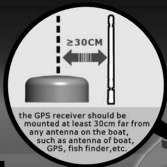
the GPS receiver should be mounted at least 30cm far from any antenna on the boat, such as antenna of boat, GPS, fish finder, etc.
